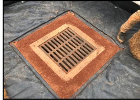
Test Setup and Installation Zone around 24-in x 24-in Inlet
