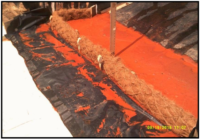
Sampling of Seepage / Retained Solids after Seepage Ends
