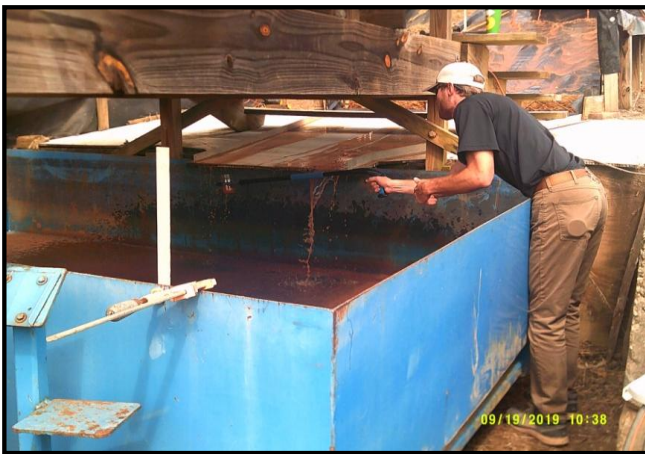
Sampling of Seepage / Retained Solids after Seepage Ends
